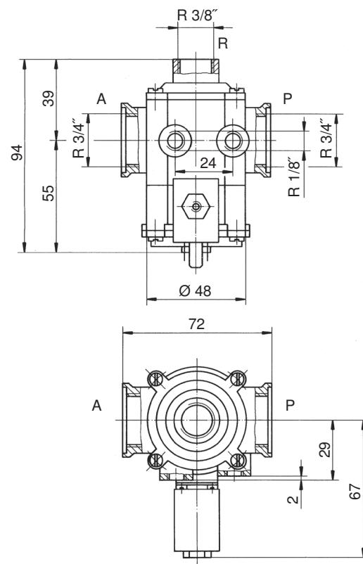
Connection R 1/8" are fitted with screw plugs as standard.
