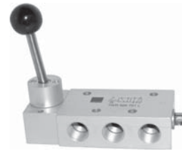
Lever actuated 5/2-way spool valve, indexed. The user can put a padlock through the 5 mm hole of the extended spool and hereby lock the valve. Temperature range: 0°C to 120°C. Seals made from FKM.
