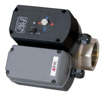
The AIR-SAVER-LS G2 can be applied on all pipe-line systems up to 2". A typical installation example is to connect the AIR-SAVER-LS to a light switch. By switching on the lights in the production area – the AIR-SAVER-LS will subsequently open. The saved compressed air flows into the factory compressed air line and the compressor kicks-in to produce the air needed to fill the system. At the end of the workshift you switch off the light(s) and the AIR-SAVER-LS will close accordingly.
