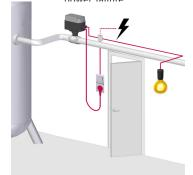
A typical installation of an AIR-SAVER-LS connected to a light switch.
