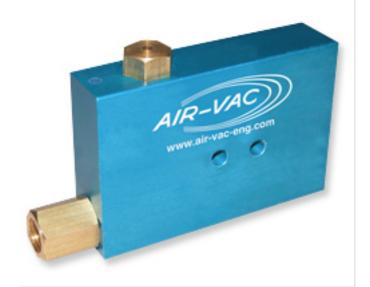
Used to evacuate chambers, degas liquids and in other processes requiring vacuum levels of 1/4"Hg absolute (8Torr). Also used as the first stage pump in applications requiring high vacuum to reduce operating time of expensive high vacuum pumping systems. Increase pumping speed above 25"Hg vacuum level.
